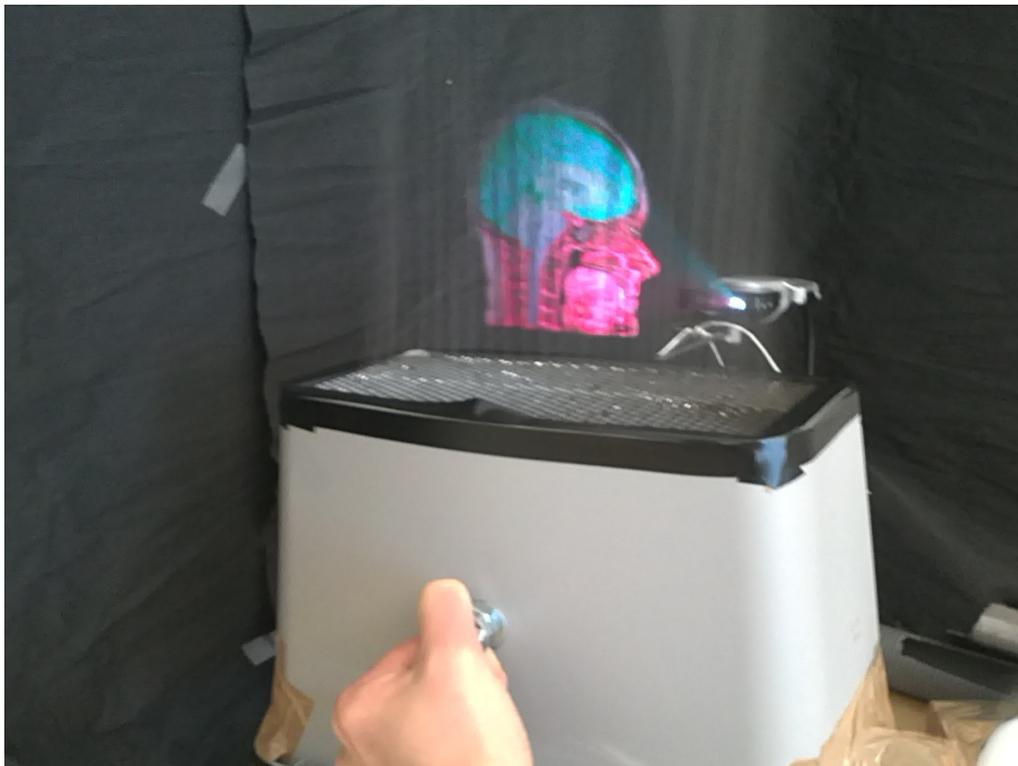
The proof-of-concept display provides an easy way to visualize volumetric objects in mid-air. The range is not as limited as with other projector-based systems, as the projector moves with the screen. Our prototype construction is still very crude, but the device can be made significantly lighter, smaller and better.
