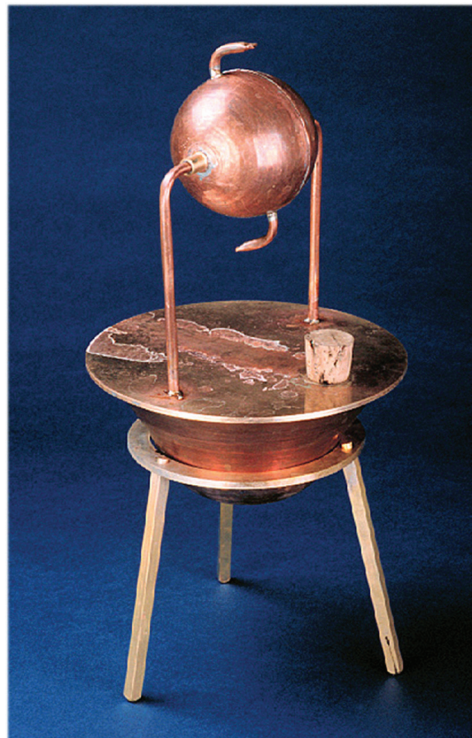
Figure 1. The aeolipile invented by the Greek Heron of Alexandria (1st century AD). It is considered the first thermal or steam engine in history and was used as a game / toy. Heron also invented the first windmill.
