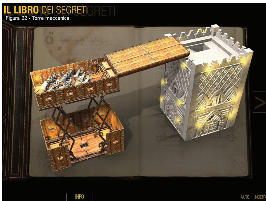
Figure 3. Extendable crane. Warriors can be raised on a wall to attack from the outside and at the same height as defending warriors on internal walls.
