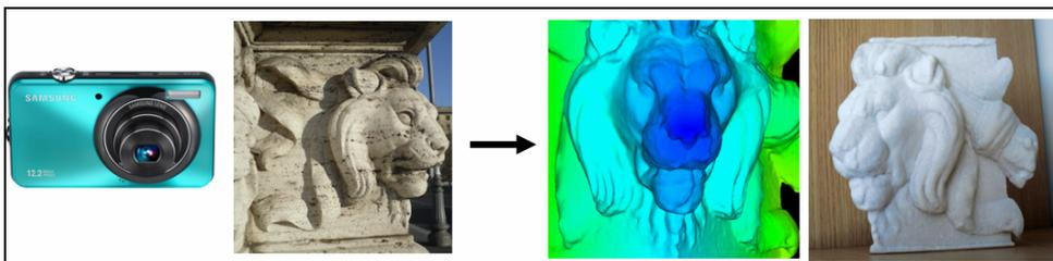
**Fig. 1.** The idea behind this work: a set of images is transformed into a 3D material replica
