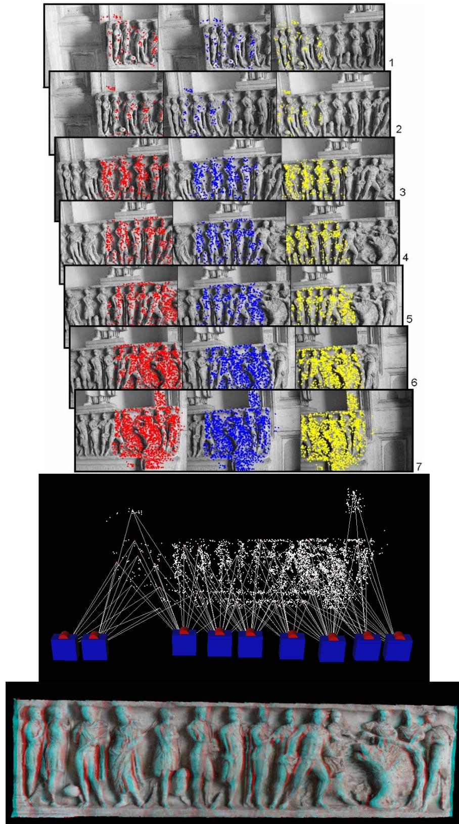
**Fig. 9.** Reconstruction of a bas-relief photographed in a famous Roman museum (Musei Capitolini): the matched image points between consecutive triplets (top), a 3D view of the camera poses (middle) and an anaglyph image of the final 3D model (bottom)
